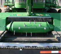
Reduce header loss and put more grain in the tank with Lankota's Grain Saver Brush Kits. Kits for John Deere® Flex & Rigid headers, mount using powerful magnets and reduces grain from getting thrown out of the head by the auger. Kits for the John Deere® Flex Drapers, are installed using existing hardware. Brush Kits reduce grain from being discharged from the head by the center feed drum and center draper belt. Lankota Brush Kits do not interfere with the operator's view of the head.
