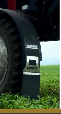
Protect your sprayer nozzles from the build-up of dirt and mud with the Lankota Mud Flaps. Stainless steel hardware secures the Mud Flap to your existing fender. Heavy-duty rubber can be cut to length for desired ground clearance. Enhance the look of your sprayer by customizing the stainless steel mounts with a name or logo.
