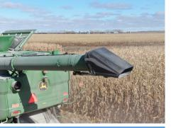
When unloading begins, the fully automated kit will automatically tip the spout to the normal unload "neutral" position. During the unloading process, the operator can manually change the angle of the spout on the fly. When unloading is complete, the spout will automatically lower to allow any remaining grain to drop out of the boot, then fully raise to the storage position.
