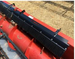
Reduce header grain loss and put more grain in the tank with Lankota's Grain Saver Brush Kits. The kit for Case IH® and New Holland® platform headers mounts using powerful magnets. The kit that fits Case IH® and MacDon® Flex Drapers is installed using self-tapping hardware. Lankota Brush Kits do not interfere with the operator's view of the head.
