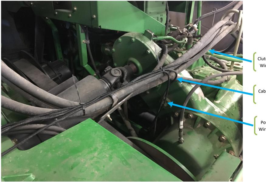
Clutch Connector Wiring Harness
