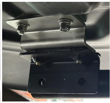
During severe suspension compression events, it is possible for the rear fenders to contact the taillights. To make this impossible, switch the taillight arms, from side-to-side, so they are higher and unable to contact the fenders.
