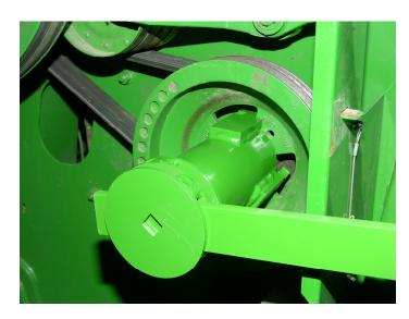
7. Remove wrench. Reinstall shield. Reinstall top feed accelerator cover. Close rock trap. Return concave to previous operating setting.
