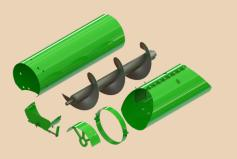
Lankota's Auger Extensions help you go further in the field. The High Unload Rate (HUR) and Non-HUR auger kits add 4 and 3.5 feet, respectively. Kits include an extension tube, saddle, flighting extension, bearing hanger, hardware and a spring-loaded Grain Saver door that restricts any dribbling of crop.
