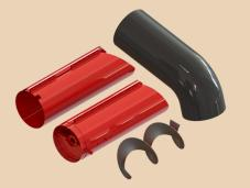
Lankota's Auger Extensions help you go further in the field. Option 1 adds almost 3 feet and includes an extension tube, flighting extension, bearing hanger, all the hardware needed and a spring-loaded Grain Saver door that restricts dribbling of the crop. Option 2 combines the tube, bearing hanger and Grain Saver door into one and includes weld-on flighting and a new spout. These kits convert the auger from bottom discharge to end discharge.
