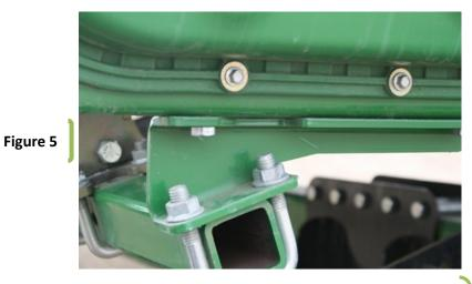
**Note:** On a 700 Series head, the front will need to be drilled. Mount the bracket with the rear hole and then use the it as a guide for the front hole.
